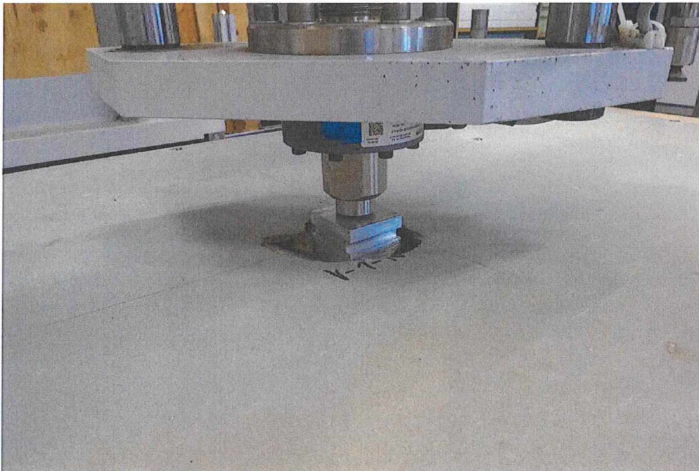
Fig. 5: Local punching failure (top view).
